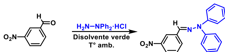
Fig. 1. Synthesis of ( E )-2-(3-nitrobenzylidene)-1,1-diphenylhydrazine through Green Chemistry.
